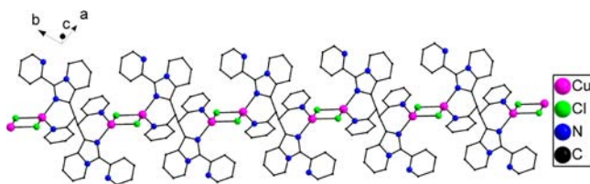
Figure 7. 1D polymeric chain of L2-Cu with alternating L2 ligand and \text{Cu}_2\text{Cl}_2 unit.
